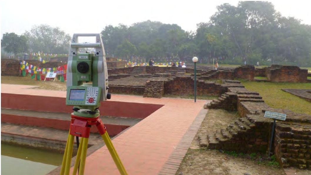
Figure 5.1. Mapping using the Leica TPS 1200. The station is controlled remotely, allowing one user to conduct the mapping rather than two.
