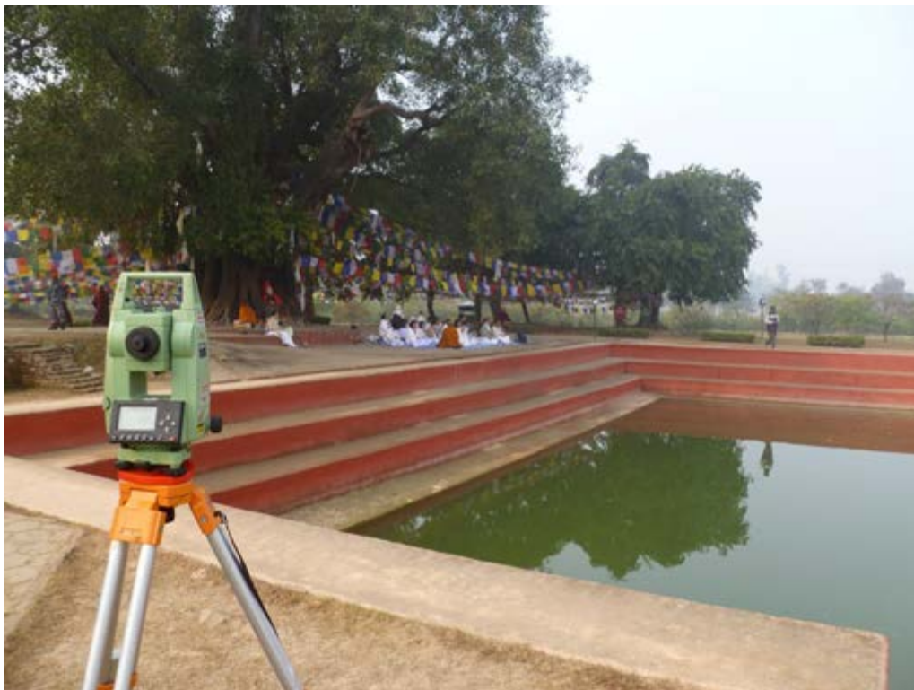
Figure 5.1. The Leica TCR307 used to map the archaeological core of the Sacred Garden in detail.
