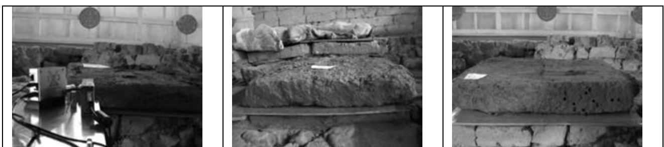
Figure 20. Performing XRF analyses on MD279 and MD280 bricks
