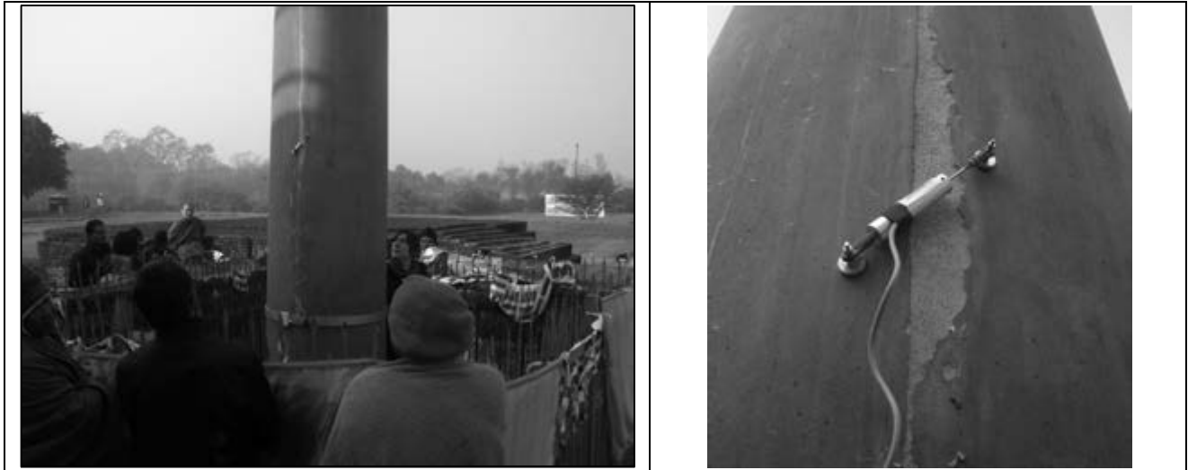
Figure 105. Strain gauge location on Asokan Pillar on February 15th, 2012
